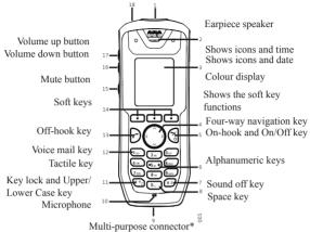
\*)Used for battery charging, software download, configuration and connection of headsets.
